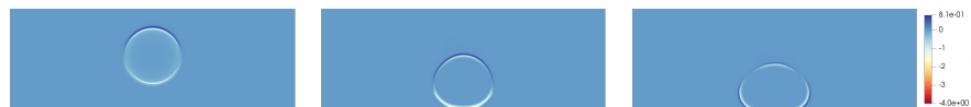
FIGURE 3. Droplet impact. Chemical potential \mu in the lower computational domain at times t = 0 , t = 0.13 , t = 0.21 .
